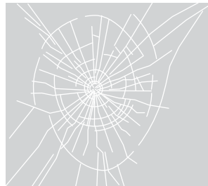
< Broken Laminated Glass >
